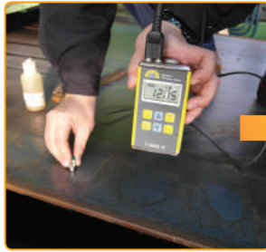
▲ Material inspection of steel coil
